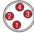
Input voltage, male, 4-pin (M8) integral connector pin-out as viewed from the end of the sensor
