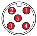
Integral D34 connector (male) as viewed from the end of the sensor
