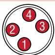
Input voltage, male, 4-pin (D54) integral connector pin-out as viewed from the end of the sensor
